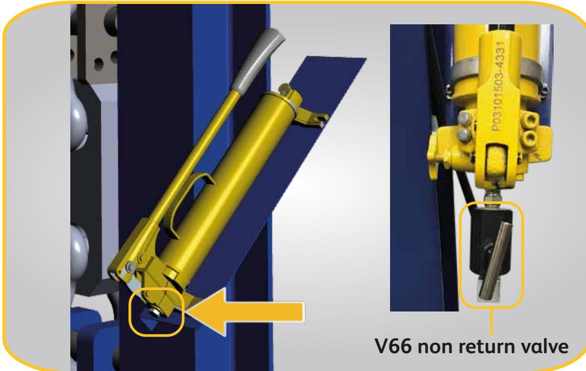
**IMPORTANT:** V66 valve has to be connected the right way round to the hand pump for hydraulic fluid to work
