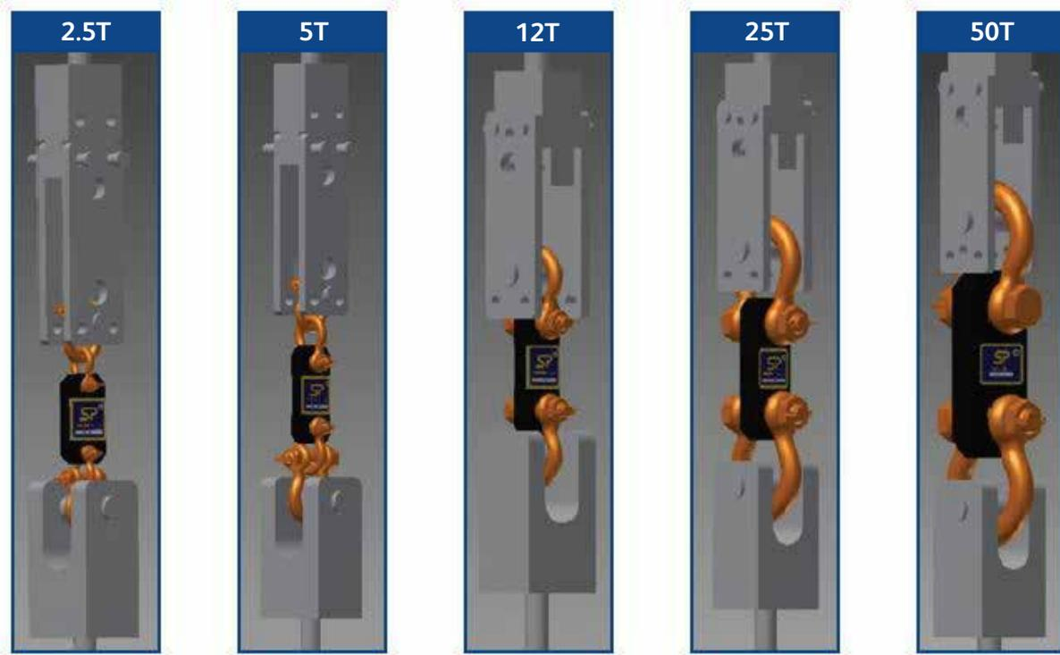
Once installed correctly, apply tension force to the load cell by pulling the hand pump's lever back and forth whilst monitoring the display on the connected HHP.
